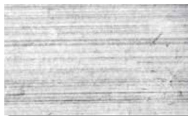
25x enlargement of the surface of a unprepared ULTRAFYLON® liner
